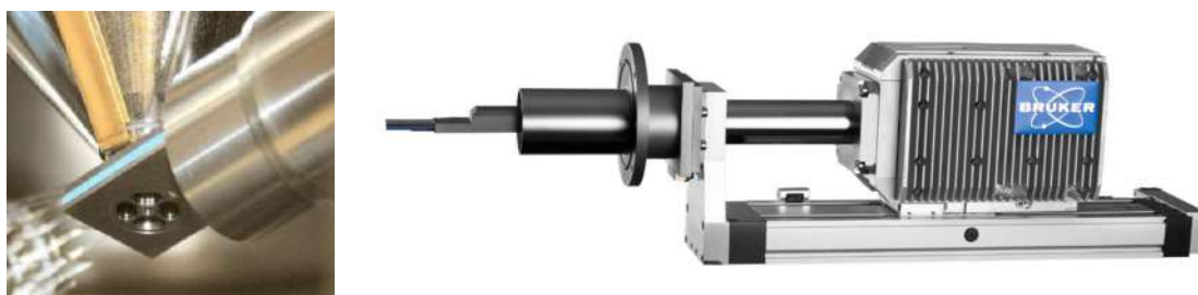
Figure 1. The XFlash® FlatQUAD detector which is positioned directly between sample and pole piece which yields a solid angle of 1.1sr.
