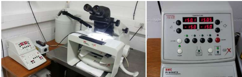
Figure 2: Cryo-ultramicrotome RMC PowerTome XL and its temperature controller indicating that a cryogenic temperature was achieved.
