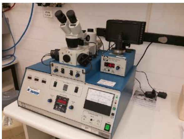
Figure 4: Gatan Precision Ion Polishing System (model 691) with a cold stage used for thinning the sample until a small hole was obtained.
