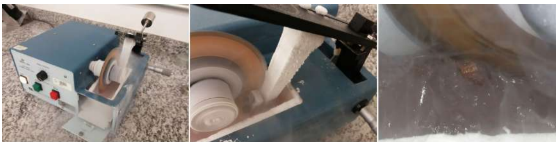
Figure 1: Cut-off machine adapted to operate cryogenically. At the right, the copper sample was being cut underneath LN. Foils of approximately 80 \mu\text{m} were obtained
