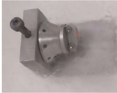
Figure 1: Cryo-rolled strip of copper attached to the cryo-ultramicrotome sample holder. Image blur due to liquid nitrogen.
