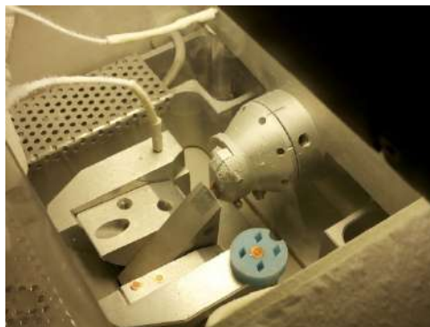
Figure 3: Cryo-ultramicrotome chamber with details on the diamond knife, sample holder with the copper strip attached and TEM grids for thermal stabilization.
