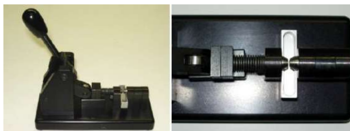
Figure 2: Disk punching tool used for obtaining a \varnothing 3mm thin disk from the thin foil.
