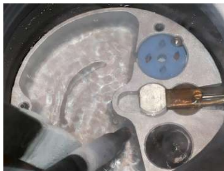
Figure 4: Details on the cryogenic transfer system for placing the grids into the TEM sample holder
